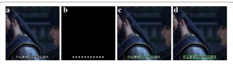
**Fig. 1** The procedure of our proposed framework: (a) The input image, (b) the outputs of character candidate classification, (c) word/character extraction after boundary expansion, and (d) the finally constructed text-line
