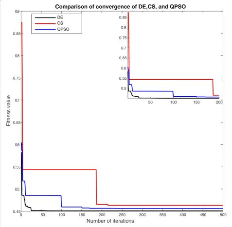
**Fig. 6** Comparison of simulation processes of QPSO, CS, and DE with W < 100 mm constraint. This figures shows the comparison of the simulation processes of the three methods with the constraint of W < 100 mm. The partial drawing at the top right corner shows the fitness function before convergence
