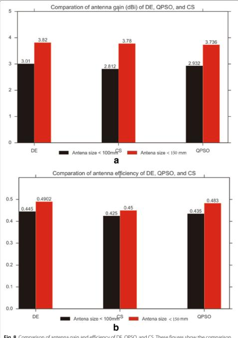
**Fig. 8** Comparison of antenna gain and efficiency of DE, QPSO, and CS. These figures show the comparison of antenna gain and efficiency of the antennas designed by the three methods with the constraint of W < 150 mm and W < 100 mm
