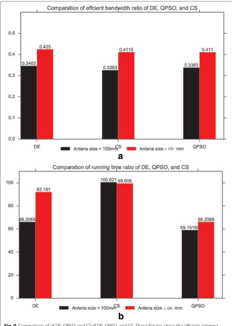
**Fig. 9** Comparison of of DE, QPSO, and CSof DE, QPSO, and CS. These figures show the effcient antenna bandwidth ratio and running time designed by the three methods with the constraint of W < 150 mm and W < 100 mm
