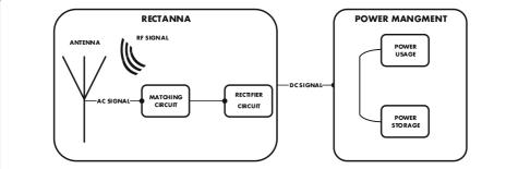
**Fig. 1** Architecture of RF harvesting system. This figure shows a typical centralized architecture of a RF energy harvesting system, including two main components: a power management component and a rectenna
