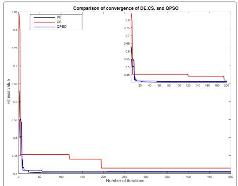
**Fig. 7** Comparison of simulation processes of QPSO, CS, and DE with W < 150 mm constraint. This figures shows the comparison of the simulation processes of the three methods with the constraint of W < 150 mm. The partial drawing at the top right corner shows the fitness function before convergence
