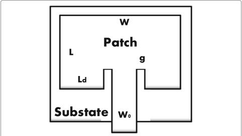
**Fig. 2** Architecture of a RMPA. This figure shows the typical architecture of a three-layer rectangular microstrip patch antenna (RMPA) with inset feed contains four geometric parameters (L, W, g, Ld)
